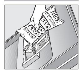
Add salt only until the reservoir is full or until water runs out of the opening. The salt reservoir holds approx. 1 kg of salt, depending on the brand used.
